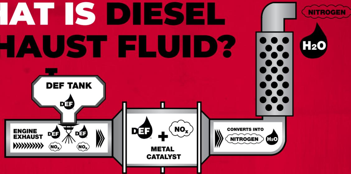
FS DEF is the clear, non-toxic, non-flammable and non-hazardous fluid utilized by the Selective Catalytic Reduction (SCR) systems to reduce Nitrogen Oxide (NOx) emissions.
